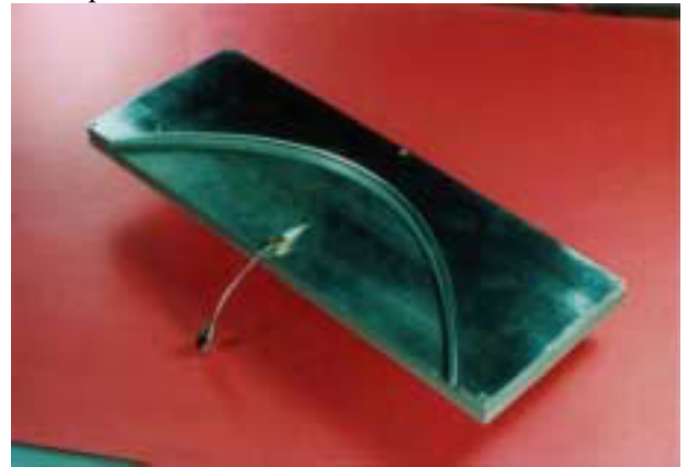
Fig. 8 Photograph of the parabolic reflector antenna fed by single radiator
